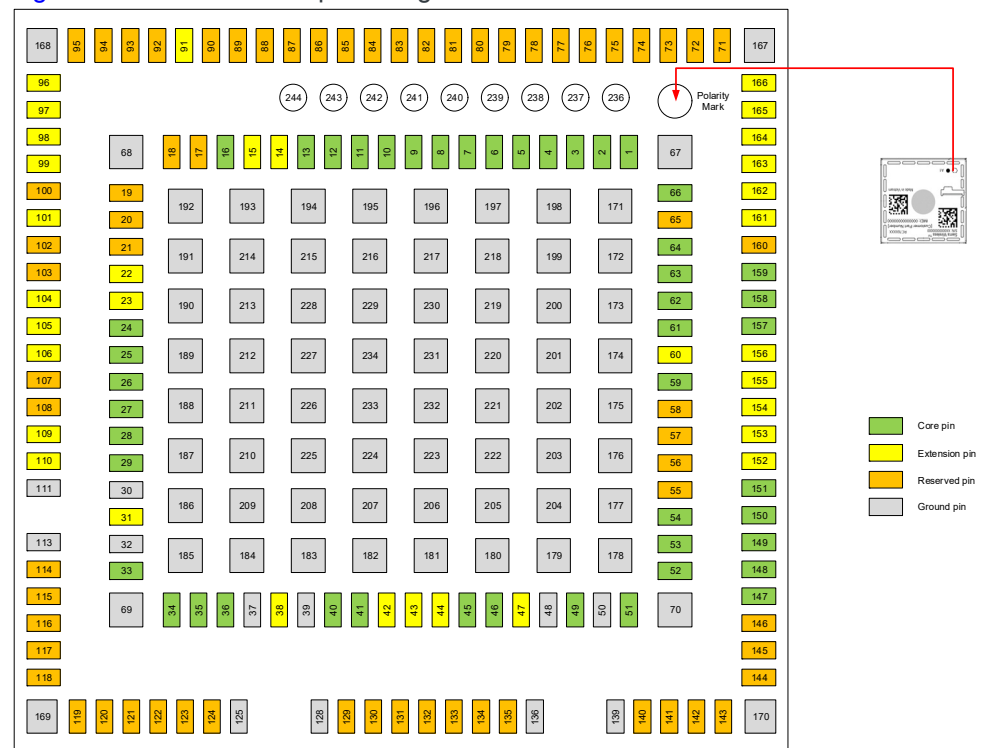
Figure 10-1: Pin Configuration (Top View, Through Module)
